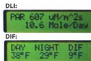
Displays Daily Light Integral (DLI) and Day/Night Temperature Difference on the LCD
