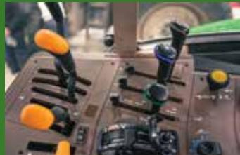
16 x 16 PowrQuad transmissions allows gear shifting without interrupting the power transmission to the wheels, which means that gears can be changed, and even reversed without using the clutch.
