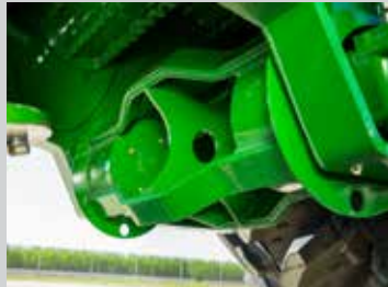
Open buttlifter options minimize soil intake and mud build-up
