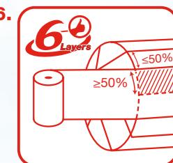
Apply at least a 50% overlap with a minimum 4 layers of film to all areas. For an optimum silage result we advise the application of 6 layers of balewrap. Where DM levels are lower than 30% or are exceeding 50%; for round bales with diameters > 1.3m; for lucerne and for stemmy crops or for square bales, a minimum of 6 layers of film should be applied.
