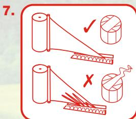
Ensure that the blade of the balewrapper's cutting mechanism is maintained in order to ensure a clean film cut after wrapping and thus avoid long film tails.
