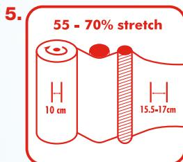
Final width of film as measured on the flat end of a round bale should, with 500mm film be 380mm-420mm, and with 750mm film be 580mm-620mm. Should film width vary outside these limits, stop wrapping and ascertain cause. Ensure pre-stretch unit rollers are regularly cleaned in accordance with wrapper manufacturer's instructions.
